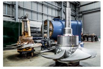
After 2 years of operation, Sydney Water had incurred significant expense in lost generation, due to partial loss of Kaplan blade functionality and early onset of internal turbine corrosion and two unsuccessful bearing repairs. Following the award of the turbine's operation and maintenance to P.E.T. and Stark, a fresh set of eyes was brought to bear on the problem. An extensive remediation program was undertaken, starting with thorough inspections, root cause analysis and options review.
