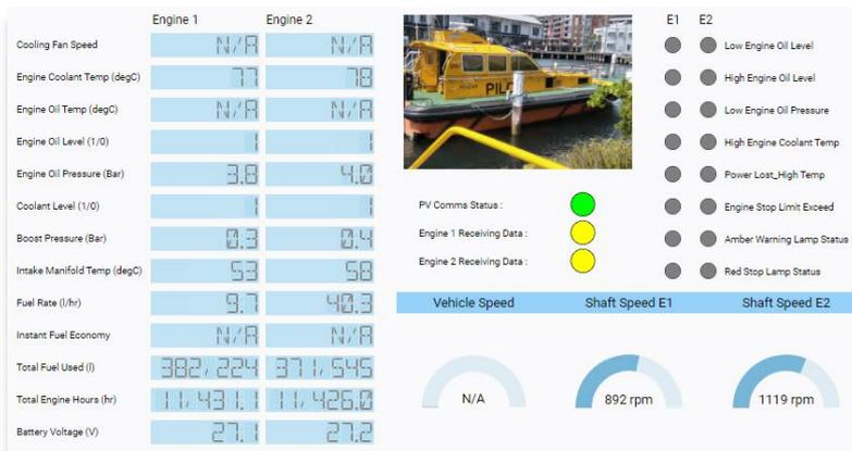
The HMI is rendered using the Perspective Engine in Ignition 8 and accessed via a web browser.
