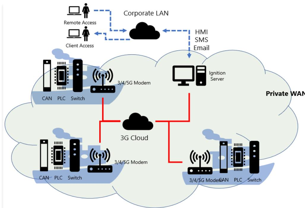
The solution had to be as **open, flexible** and as **extendable** as possible, using off the shelf components. While the initial role out was across SCANIA DI16 marine engines the solution had to cater for different engines models and makes. The solution could not interfere with engine control and should be as passive as possible.
